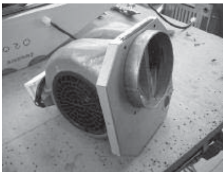
4. Position internal flange over blower housing.
