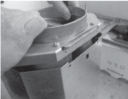
8. Place blower with attached flange into motor housing as shown on Fig-A.
